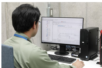
Monitoring screen of the device management system installed in the plant control room. The operating status of field devices can be checked from the control room without going to the field.
