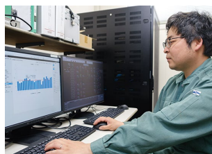
Monitor screen of EneSCOPE for EMS (left) and the Harmonas-DEO harmonized automation system introduced as the DCS*1 (right), installed in the server room.
