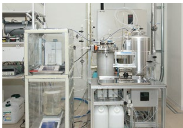
Micro liquid flow standard device. It measures weight and time with high accuracy, such as the minute flow rate of liquid (g/min) that would take 5 minutes to fill a teaspoon. This standard device was developed by Azbil.
