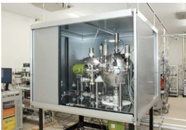
Vacuum generator (expansion method device). Applying Boyle's law, it generates a highly accurate vacuum of around 1 to 1000 Pa (1/100000 to 1/100 of atmospheric pressure). This standard device was developed by Azbil.
