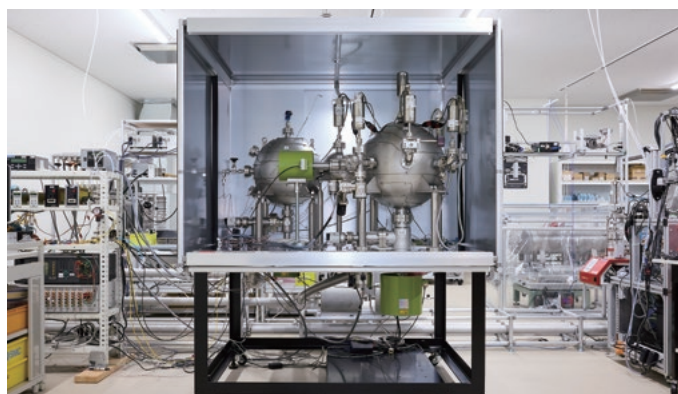
Calibration office at the Fujisawa Technology Center and a (center) high-precision vacuum calibration system
